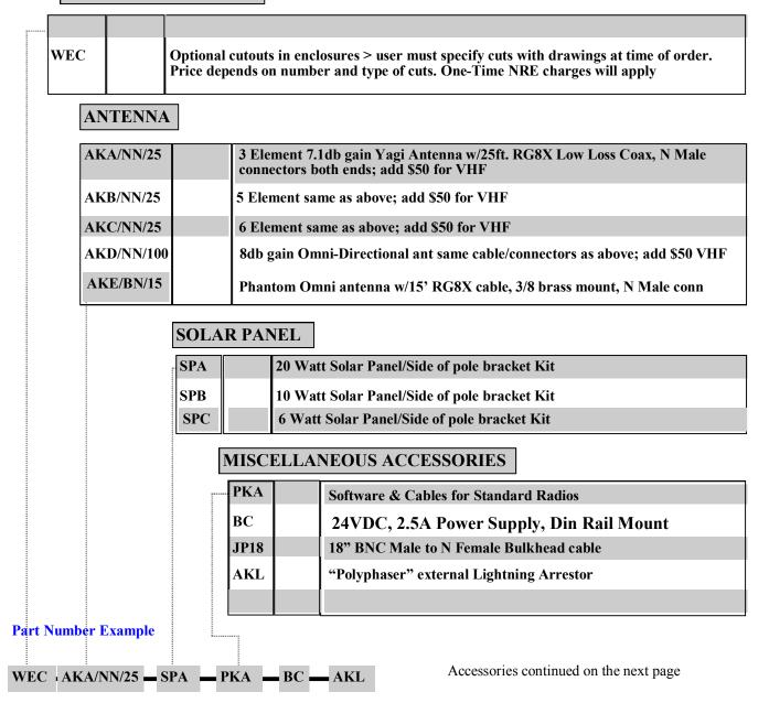
With Window Kit, 3 Element YAGI Antenna, 20 Watt Solar Panel, Radio Programming Kit, Power Supply, External Lightning Arrestor
